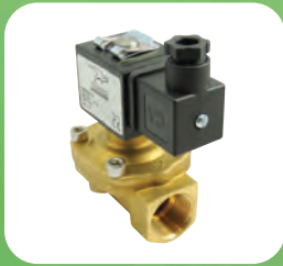
211 Électrovannes à commande directe (1/4") ou mixte (3/8" à 1") - 2/2 2/2 - Direct acting (1/4") or Zero pressure diaphragm controlled (3/8" to 1") solenoid valves
